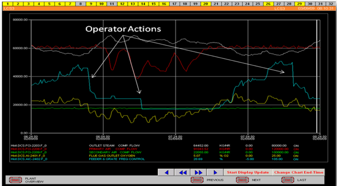
Figure 2, typical control problem
