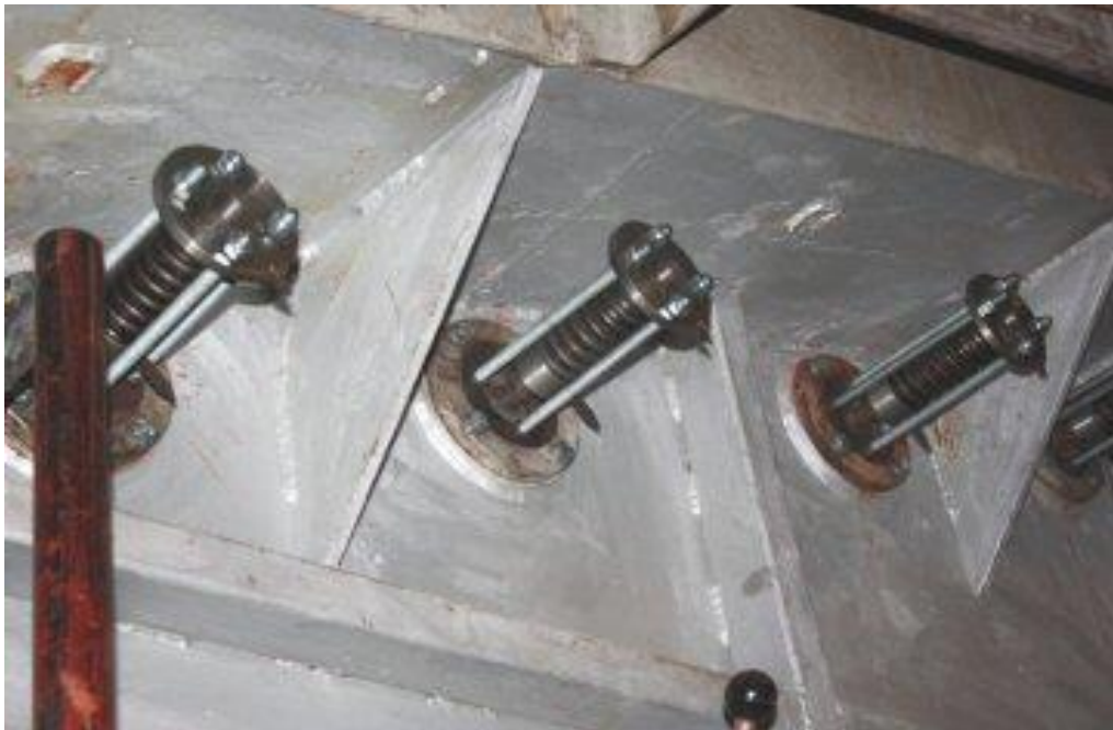
Photo 9 the well proven spring loaded Dublix lateral adjustment system is normally applied to the DUB 3 grate carpet
