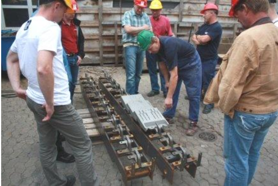
Photo 4 careful inspection of the details in the DUB 3 grate carpet
