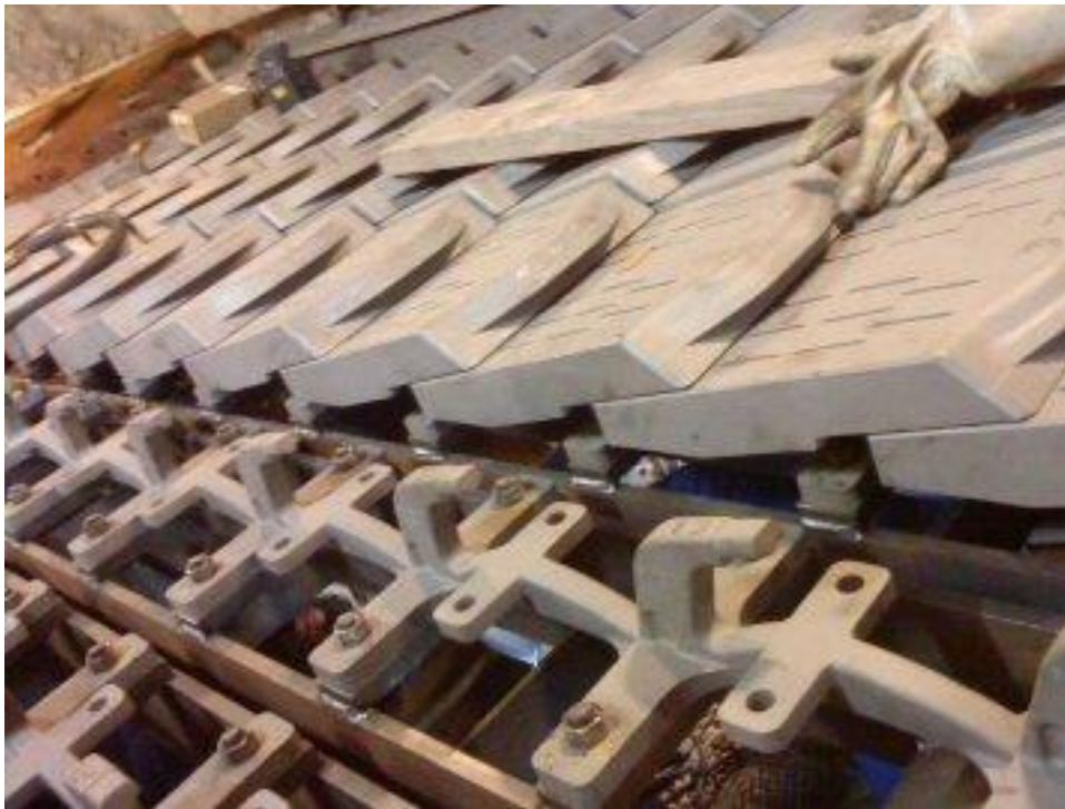
Photo 7 details from an installation showing the earlier hook fastening system, protected from the heat exposure under the grate surface
